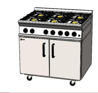
When comversion is complete addix new data label and gas type label supplied with the conversion kit, detailing type of gas and pressure.
